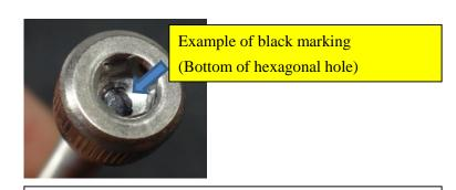
HANARL is applied to the area from the head of the bolt over a range of about 10mm along. It looks whitish. Additionally, there is black marking on the bottom of the hexagonal hole.
