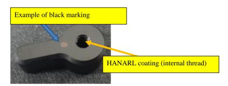
HANARL is applied to the internal thread.
