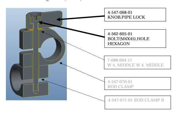
(Old) KNOB,PIPE LOCK 4-547-068-01 (New) KNOB ASSY (SVC), PIPE LOCK A-2196-367-A
